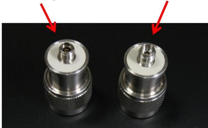
All adapters must be kept clean and undamaged to maintain measurement accuracy. Adapters should be regularly cleaned, and damaged adapters replaced.
