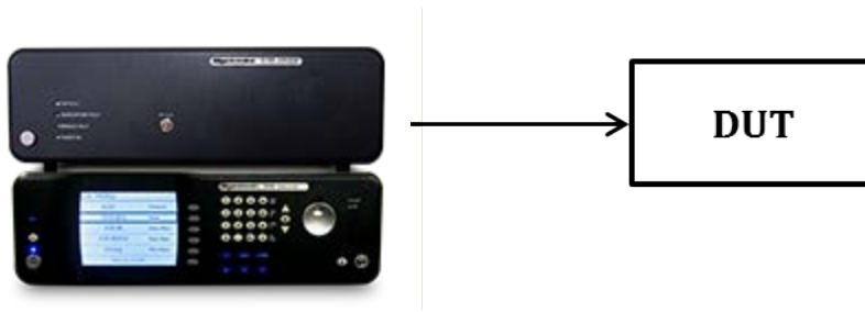
Figure 1) Signal generator and amplifier driving a device-under test (DUT)
