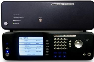
GT-1000B 20 GHz Microwave Power Amplifier and 2520B Microwave Signal Generator
