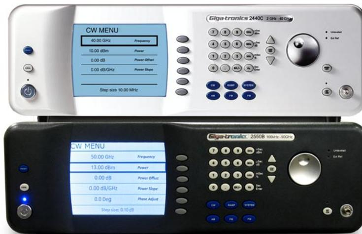
The Giga-tronics Model 2400 and 2500 Series Microwave Signal Generators are designed with several types of memory. The user-accessible memory is used to store various parameters pertaining to the synthesizer configuration, which include frequency, level parameters set by the user. There are 10 user-accessible memory locations for storing instrument states and 1 additional location reserved for recovering the last instrument state automatically stored when the synthesizer is powered down.
