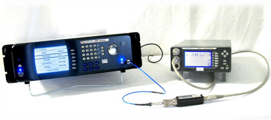
Figure 6. External Cable Loss Correction Factors can be stored in the 2500B
