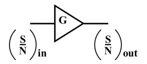
An amplifier with gain G and noise figure defined in terms of signal-to-noise ratio:
