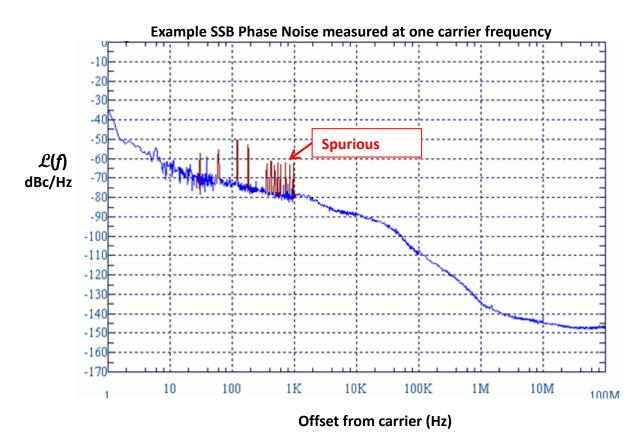
The above example is a typical log-log plot of signal generator phase noise, as measured on a phase noise test set. The vertical axis is amplitude relative to the carrier, which is not shown. The horizontal
