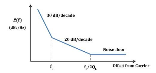
From the model (Leeson's equation), it can be seen that the phase noise of an oscillator can be reduced by the following:
