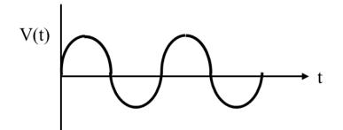
In the frequency domain, an ideal sine wave signal is shown as a single frequency in the spectrum.
