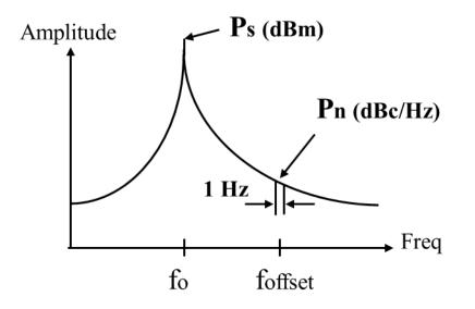
Measured directly on a microwave spectrum analyzer,  $\mathcal{L}(f)$  is the ratio of the noise power in a 1 Hz bandwidth, at a specified offset from the carrier, to the carrier signal power.
