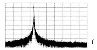
It is important to point out that the amplitude noise and phase noise are small perturbations. The goal in signal generator design is to have these as small as possible, from at least 40 dB less than the carrier to as much as 170 dB less than the carrier, limited only by the kTB thermal noise floor.
