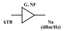
$$Na = NF (dB) + G (dB) + kTB (dBm/Hz)$$
